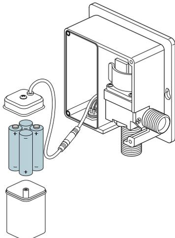
**3. Reinstall Battery Box & Control Box Cover**
