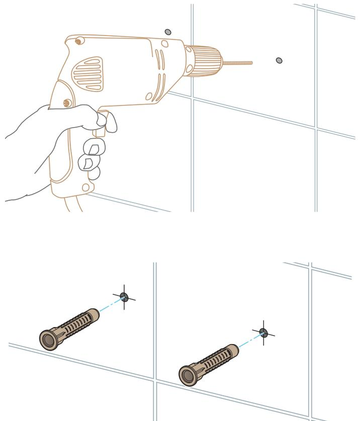
**4b.** Mount the control box on the wall. Drill two 1/8" (3mm) holes as shown, and push drywall anchors into each hole. Secure the control box to the wall with the drywall screws.
