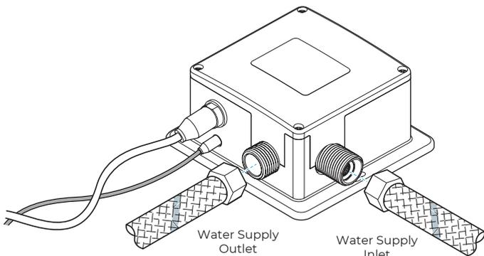
Please wait approximately 60 seconds after connecting the sensor cable for sensor calibration to complete and to begin using the faucet.
